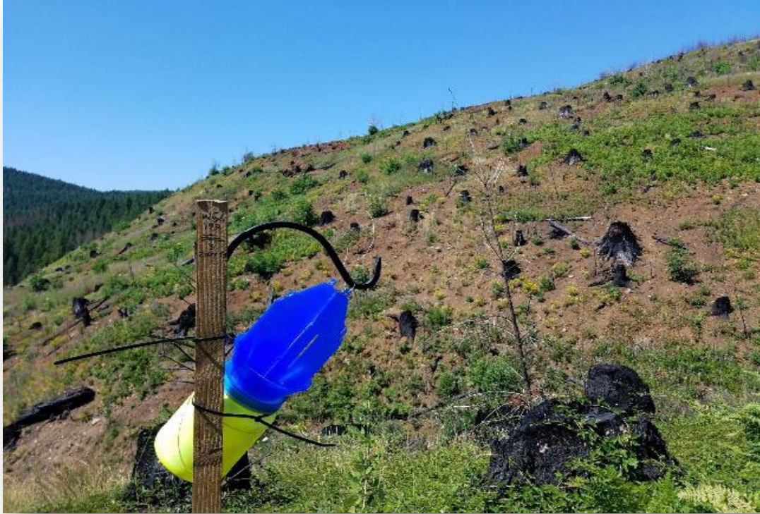
Figure 5. Blue vane traps, brightly colored fluorescent yellow and blue to attract bees, were placed on gardening Shepard's hooks and reinforced with a labelled stake. We tilted the device at a 45-degree angle to reduce any likelihood of excessive rain flooding the trap as per suggestions by Lincoln Best and the Ponisio lab. Photo by Tim Lawes.
