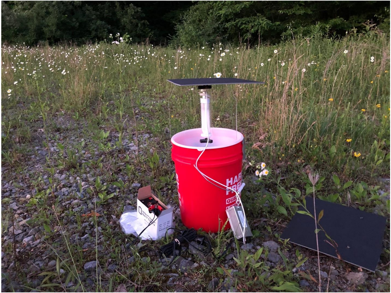
Figure 5. In-field example of black-light traps that were used to collect specimens. Traps were comprised of a 5-gallon bucket, altered funnel, 12 W black light, three acrylic panes, small battery and electronics. At the bottom of the funnel, a 1-gallon bag was attached to both collect specimens and to discourage escape.
